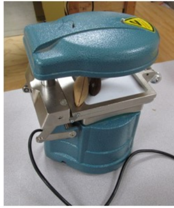
Chuck Stroble demonstrating his vacuum forming machine
